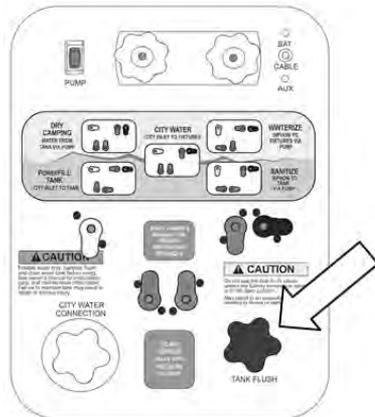
**Sewer Tank Flush Inlet on Utility Center**
